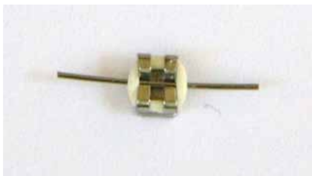
Figure 1. Fragment of orthodontic appliance (metal bracket, elastomeric module, Ni-Ti round wire)
